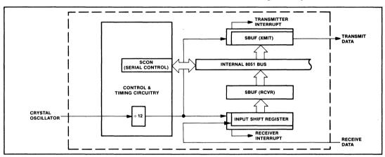
Figure 2.6.A Serial Port - Synchronous Mode 0
